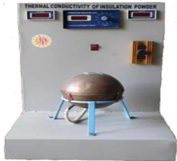
Fig 5. (a) Location of Thermocouples in Spherical Shell; (b) Apparatus of Thermal Conductivity of Insulating Powder
