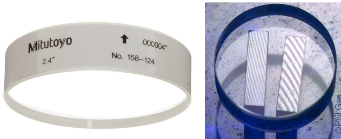
Fig. Optical flat and its use over slip gauges to test the flatness of the surfaces
